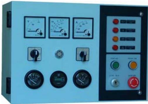
**Baifa Standard Control Panel** is the basic configuration for normal operation and usage, it is of some advantages such as easy to operate, various function and well protection. Operative buttons such as Turn On, Per-heat, Starting, Stop (Emergency Stop) on the panel. While malfunction occurs, control panel will stop the generator and also alarm with light or buzz.
